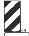
12" x 24" Vertical Panel mount with diagonal strips sloping down towards travel way
