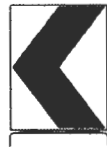
18" x 24" Sign (Maximum Sign Dimension) Chevron CB-1a, Opposing Traffic Lane Divider, Driveway sign D70a, Keep Right R4 series or other signs as approved by Engineer
